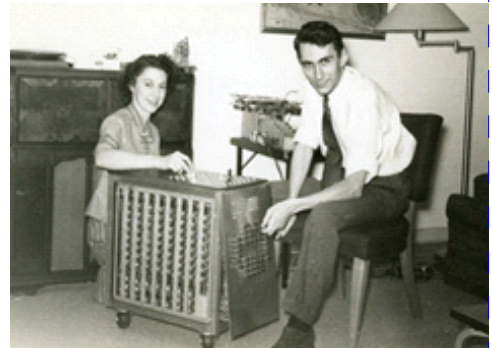
Shannon built this chess-playing machine, an ancestor of Deep Blue. It could play six moves of an endgame. Photo courtesy of the Shannon family
